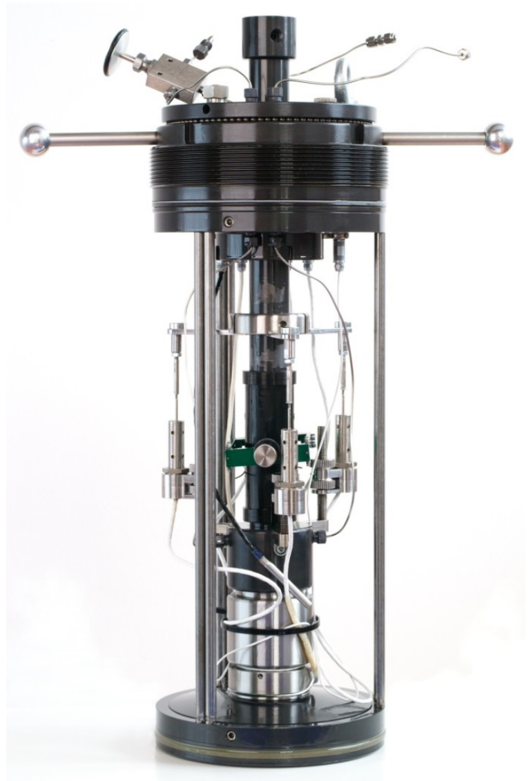
Triaxial cell set up for the measurement of both, axial load as well as axial and radial deformation
